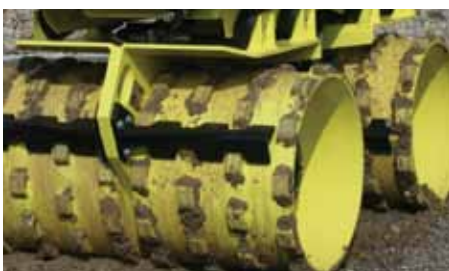
2 drum widths 63 cm or 85 cm
