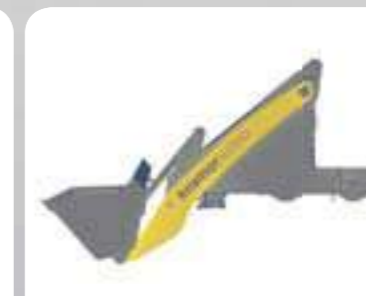
Maximum tip-back angle for safe loading transport.
