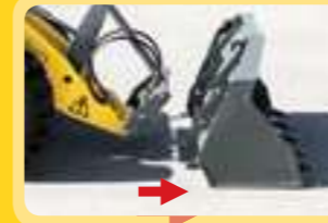
1 Easy to drive up to tool attachment.
