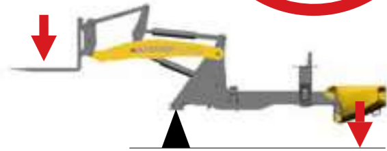
Constant leverage for constant payload.
