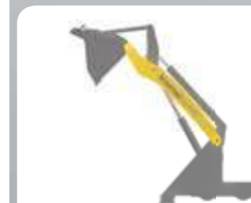
Broad dumping angle for simple emptying of bucket.
